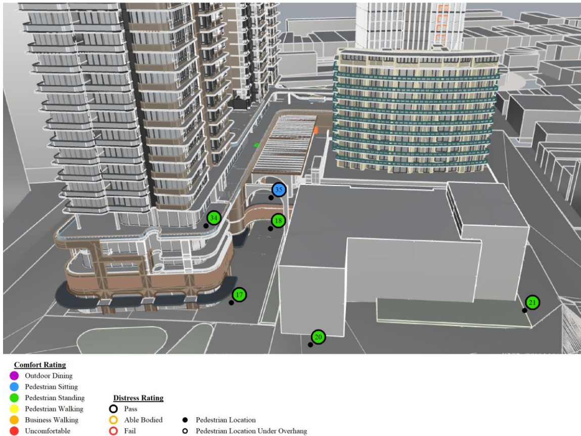
Figure 7: Pedestrian wind speed measurement locations with comfort/safety ratings – Ground/Podium Level – North Isometric view.
